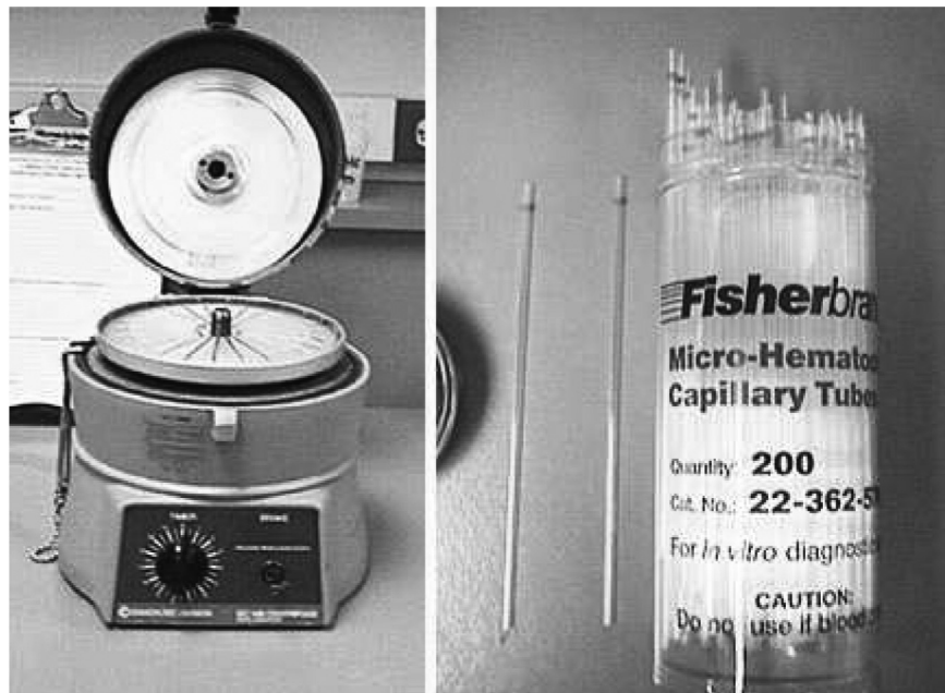
Fig. 4.1: Capillary tubes (right) and the microhematocrit centrifuge (left)
