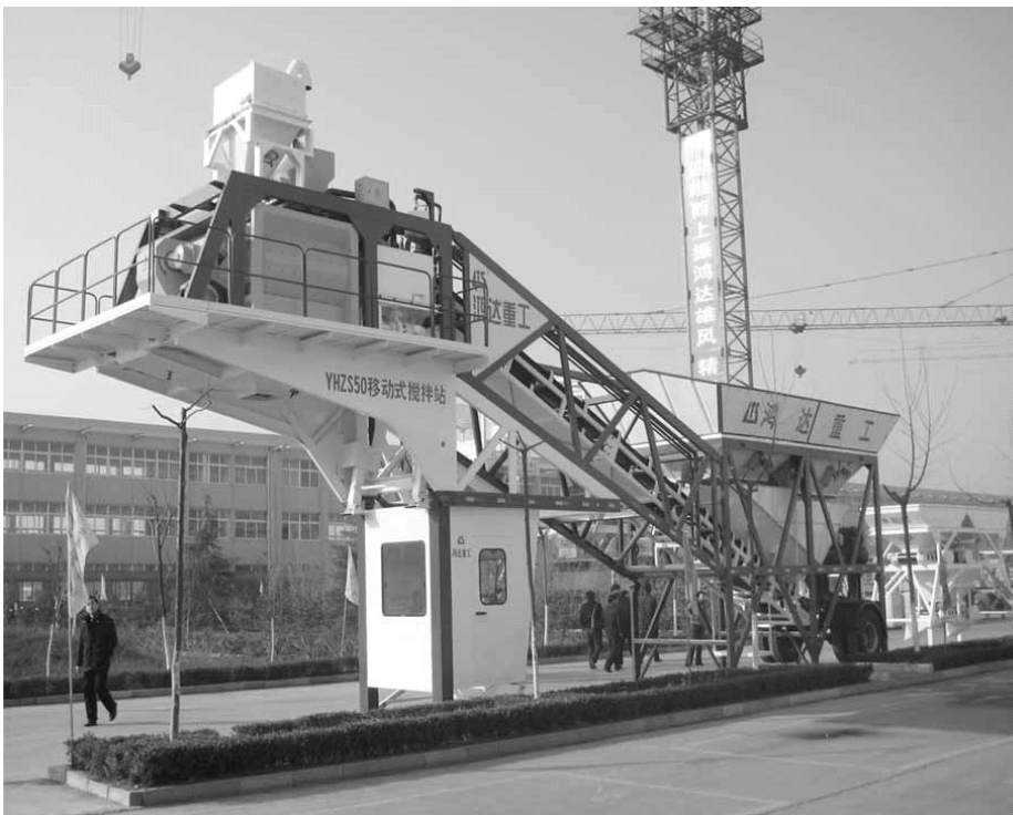
Fig. 10.1: Mobile Mixing Plant
